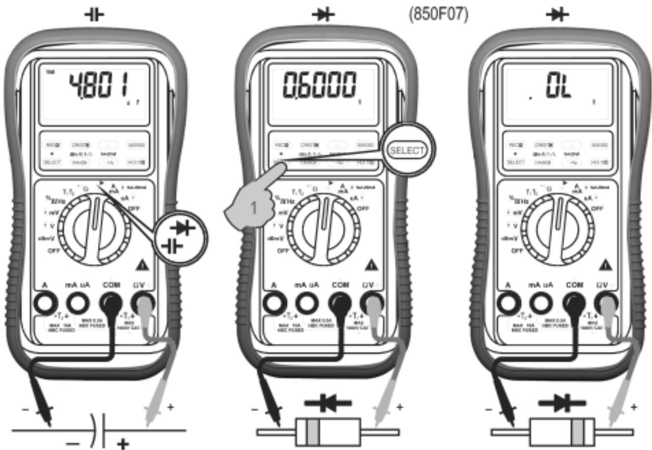
Note: Normal forward voltage drop (forward biased) for a good silicon diode is between 0.400V to 0.900V. A reading higher than that indicates a leaky diode (defective). A zero reading indicates a shorted diode (defective). An OL indicates an open diode (defective). Reverse the test leads connections (reverse biased) across the diode. The digital display shows OL if the diode is good. Any other readings indicate the diode is resistive or shorted (defective).
