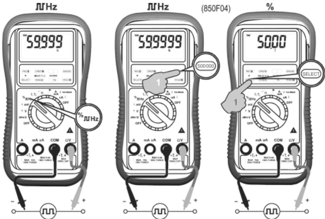
Note: Unlike the Line Level Frequency measuring function as previously stated, this Logic Level Frequency function is set only at the highest input sensitivity to measure digital type electronic signals.
