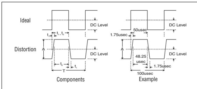
**Figure 3 Waveform Distortion**
