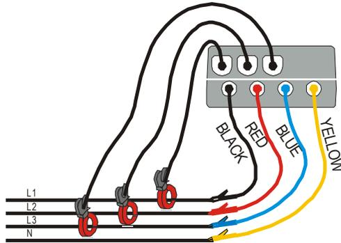
Instrument connection in a three-phase 4 wire system
