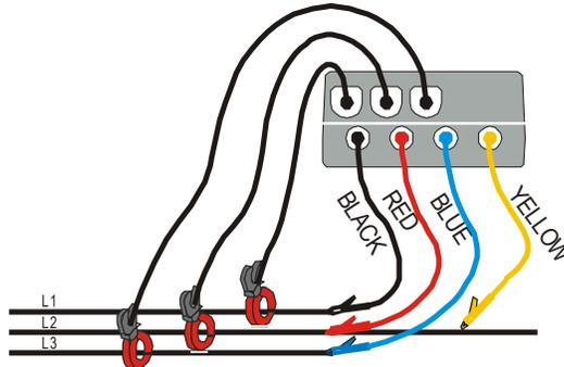
Instrument connection in a 3 wires three-phase system
