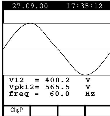
Example of screen in "3 wires" three-phase system
