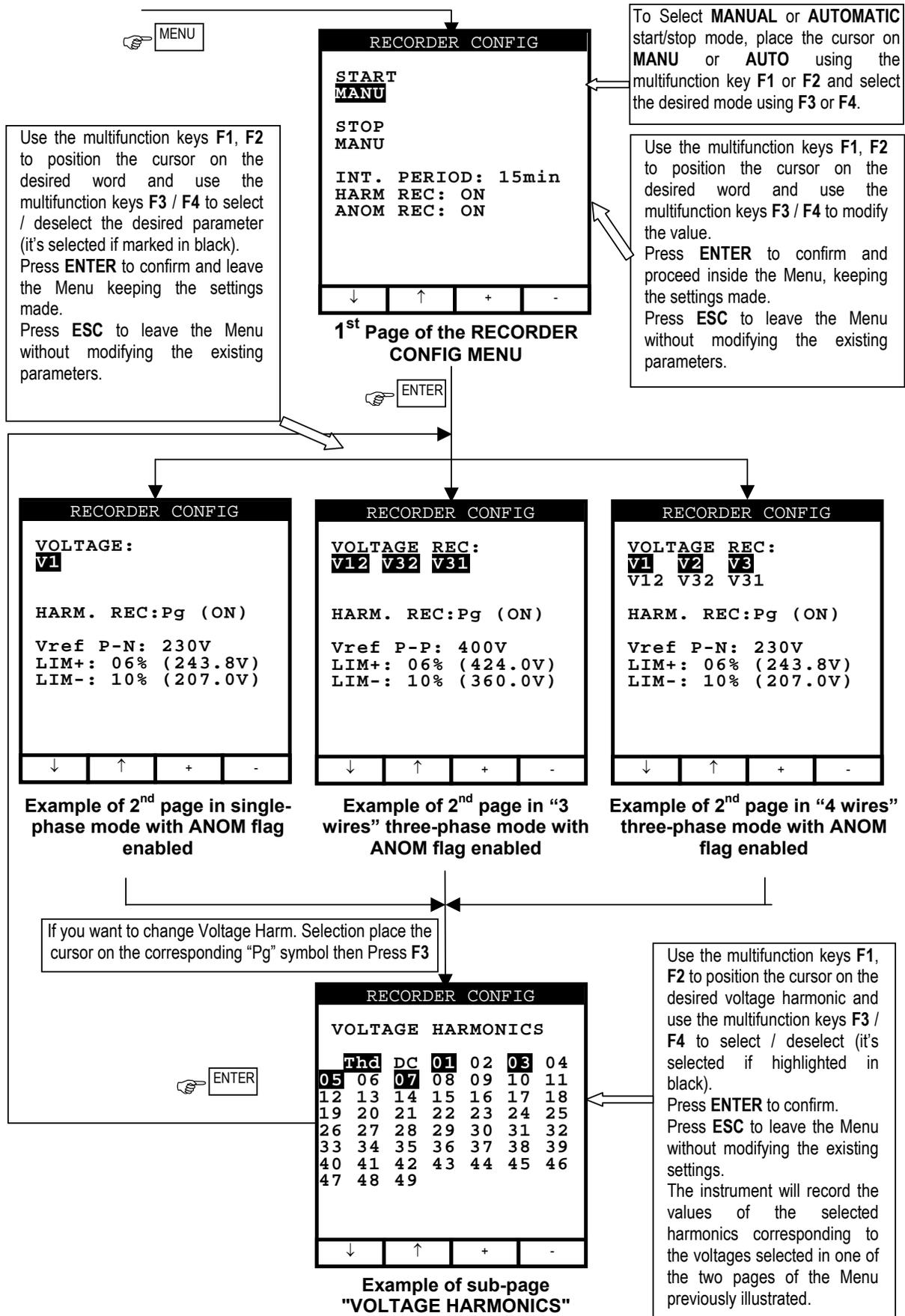
Use the multifunction keys **F1**, **F2** to position the cursor on the desired word and use the multifunction keys **F3 / F4** to modify the value or select / deselect the desired parameter (it's selected if marked in black). Press **ENTER** to confirm. Press **ESC** to leave the Menu without modifying the existing settings.
