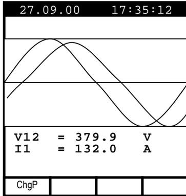
Example of screen in "3 wires" three-phase mode
