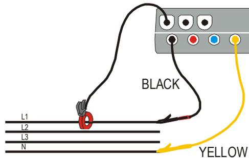
Instrument connection in a single-phase system
