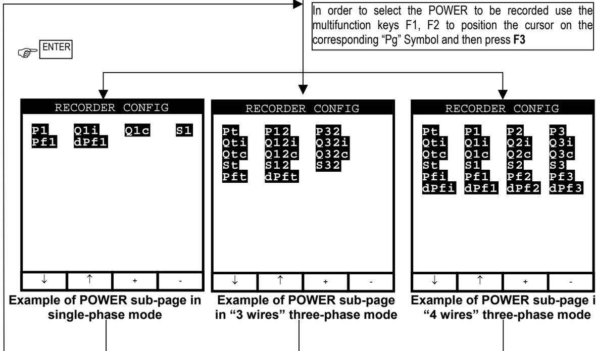
Selecting the active powers for the recording, the corresponding active energies will be automatically selected.
