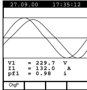
Example of screen in "4 wires" three-phase mode
